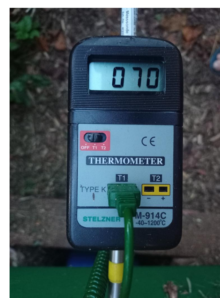
Thermophilic temperatures (50-70°C) are reached at the core
